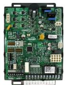
sends a description of the unit to the optional **icomfort Touch™ Communicating Thermostat** to automatically configure the number of stages and features available.
