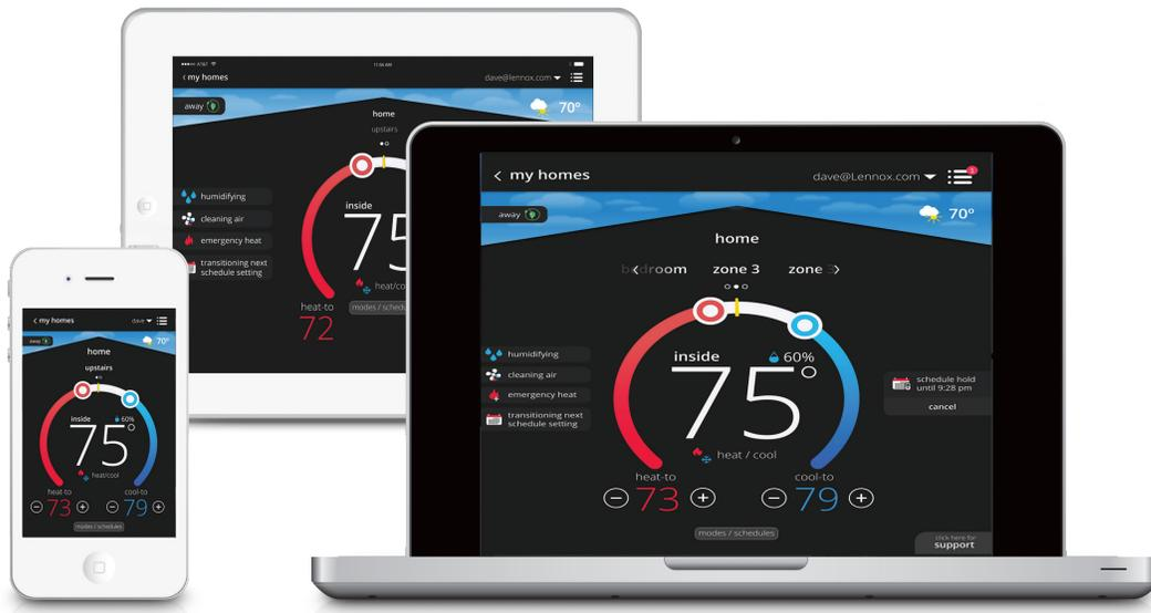
Wi-Fi remote temperature monitoring and adjustment through a home wireless network via desktop PCs, laptops, and apps for smartphones or tablets.
