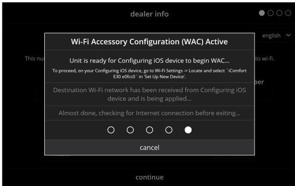
After power is applied to the thermostat for the first time, it displays the iComfort® “splash screen” (see page 24), then the Wi-Fi Accessory Configuration (**WAC**) Active screen for configuring the IOS device will appear on top of the dealer info setup screen.
