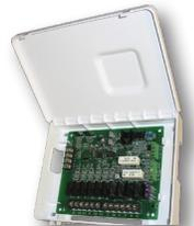
**ATTENTION** - The Lennox iComfort® S30 Ultra-Smart thermostat with Equipment Interface Module (EIM) will work with most 24VAC furnaces, air conditioners, air handlers and heat pumps (up to 3 stages of heat and 2 stages of cooling), EXCEPT it will NOT work with any brand of communicating HVAC equipment other than LENNOX®.
