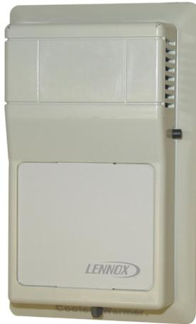
Two-wire non-communicating wall-mounted zone sensors. Each sensor is designed to fit a single gang electrical handy box. The COSNAJ01AE1- has a sensor offset slide that allows for easy temperature adjustment. Each sensor also has SysBus/ZoneBus phone jack that may be connected to the network. The bus connection is not required for sensor operation.
