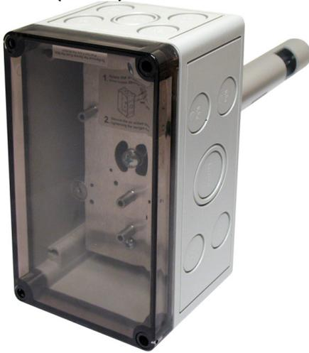
Converts standard wall-mount CO<sub>2</sub> sensors to duct mount applications. The custom internal mounting bracket secures the base of the sensor inside the aspiration box. Power is applied by running conduit through a knockout and wiring to the terminal blocks located on the sensor mounting bracket. The enclosure is lightweight, durable, and can be installed in minutes.
