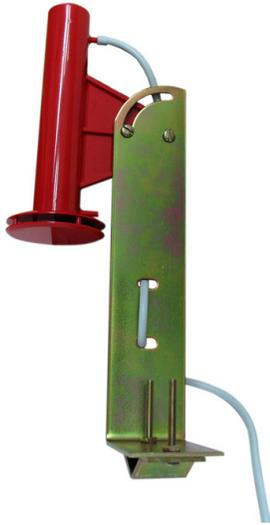
The Outdoor Air Weather-Head effectively reduces the fluctuation of outdoor static pressures caused by wind gusts. Eliminating this fluctuation is necessary in the control of building pressures which use outdoor static pressure as a reference.
