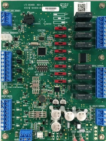
The **Building Controller** is used for controlling lights, vent hoods, exhaust fans, sprinklers and other devices based upon unit occupied operation or time schedule for the iCON Building Automation Solution. It also allows many other interactions between the building and the HVAC equipment such as load shedding, wake up/shut down building switch and overrides based on temperatures and/or analog inputs. The Building Controller requires the iCON Local Display for system control.
