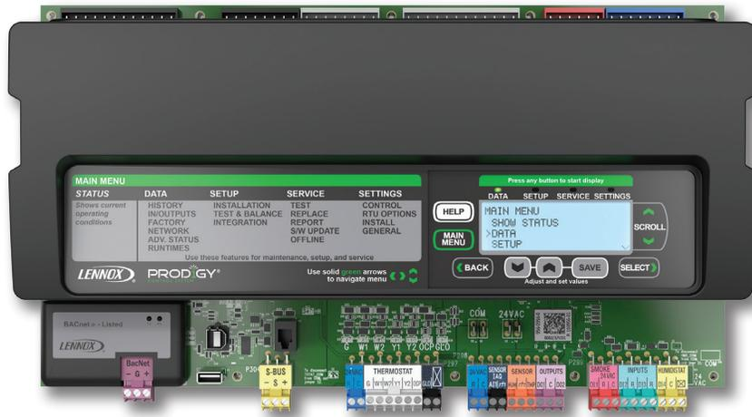
The Prodigy 2.0 Unit Controller is a microprocessor-based control board that provides flexible control of all unit functions.
