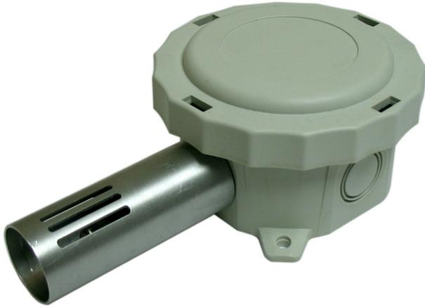
Outdoor temperature sensor used primarily with the Building Controller and Network Thermostat Controller. It has a water-proof plastic wiring enclosure. The temperature sensor is surrounded by a vented aluminum enclosure to reduce the effect of wind and sunlight on the temperature measurement.
