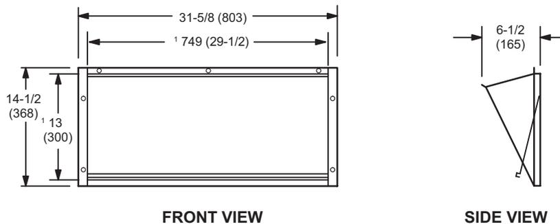
NOTE - Opening size required in return air duct.
