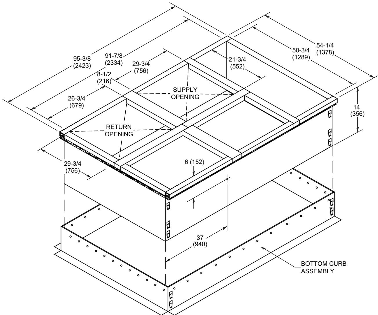
NOTE - Maximum slope pitch is 3/4 in. per 1 foot (19 mm per 305 mm) in any one direction.
