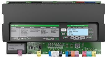
controller is a microprocessor-based controller that provides flexible control of all unit functions.
