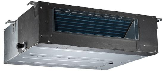
Slim, compact design for limited space requirements. Installs out of sight between the drop ceiling and ceiling slab with ducted distribution to the indoor space.
