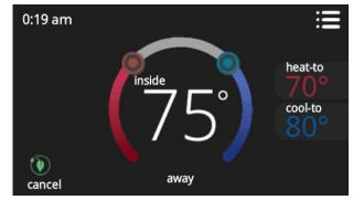
Set heating or cooling setpoints during unoccupied periods.
