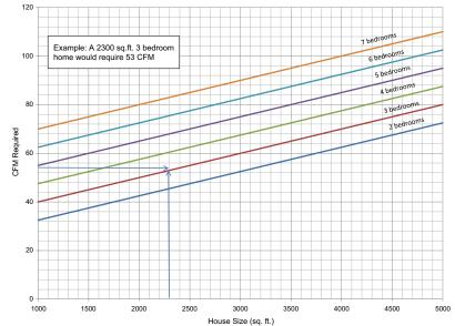
Step 2 - Determine How Much Ventilation Air the System will Deliver
