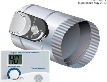
extreme hot, cold or humid air from being used to ventilate the house. The Digital Ventilation Controller prevents ventilation operation when indoor relative humidity is above 55% and the outside temperature is above 50°F to prevent excess indoor humidity levels.
