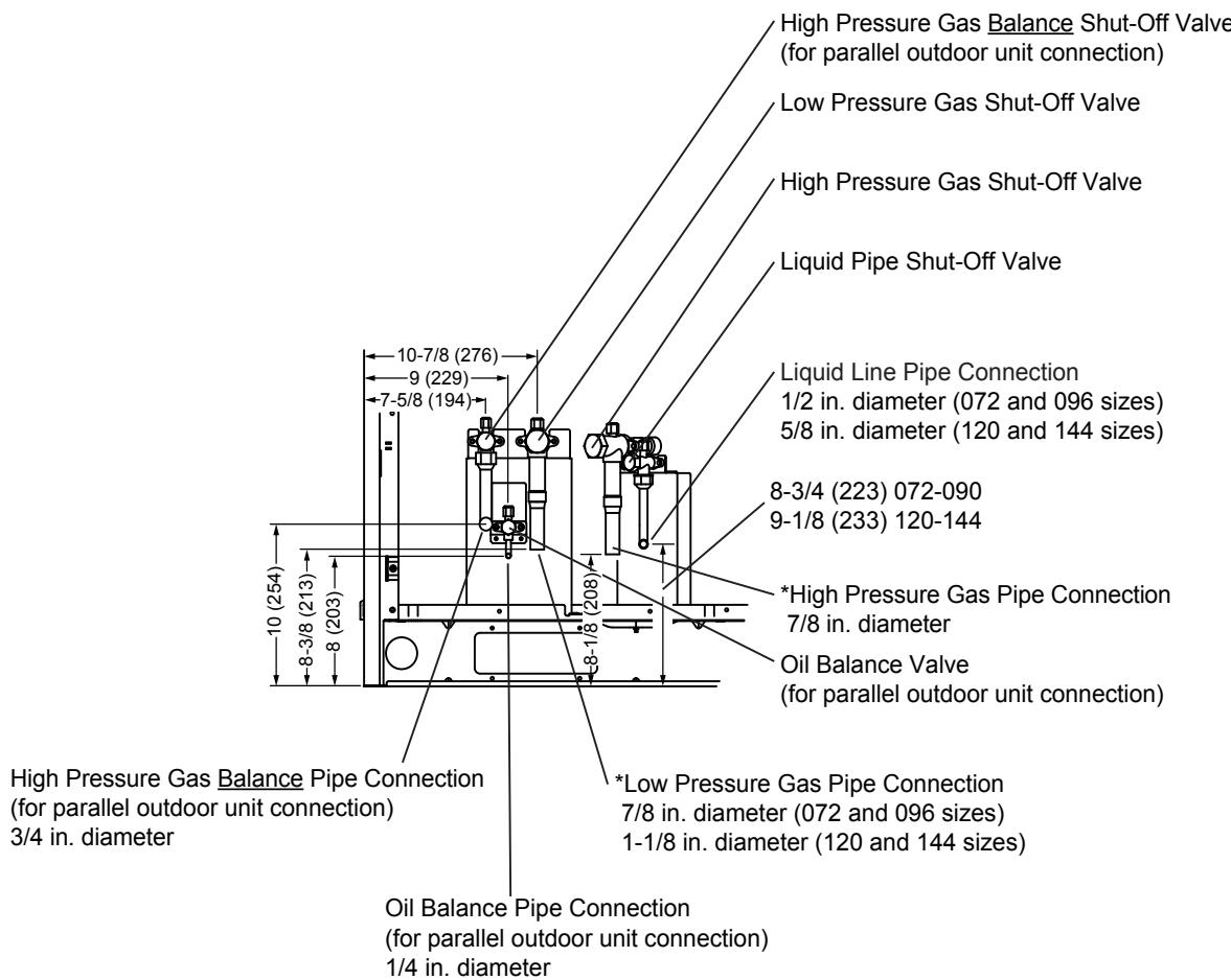
\*NOTE - Two 90° Elbows are furnished for Low Pressure and High Pressure Gas Pipe Connections from the front of the unit.
