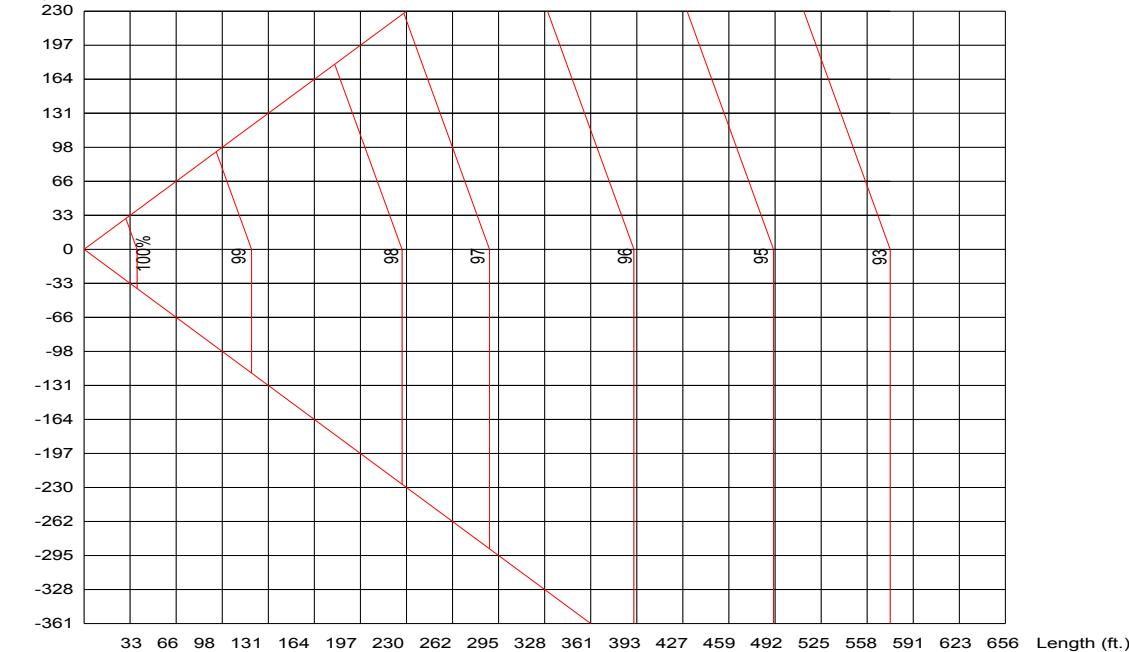
L = Length of equivalent refrigerant pipe.
