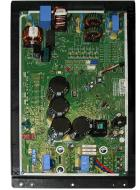
Power Factor Correction (PFC) circuit monitors the DC bus for high, low and abnormal voltage conditions to protect the compressor.
