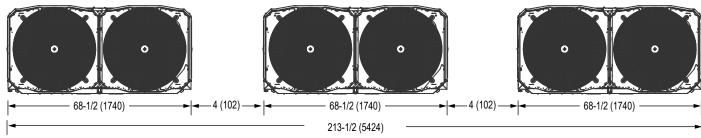
**NOTE** - All the outdoor units manifolded together should be installed at the same elevation.
